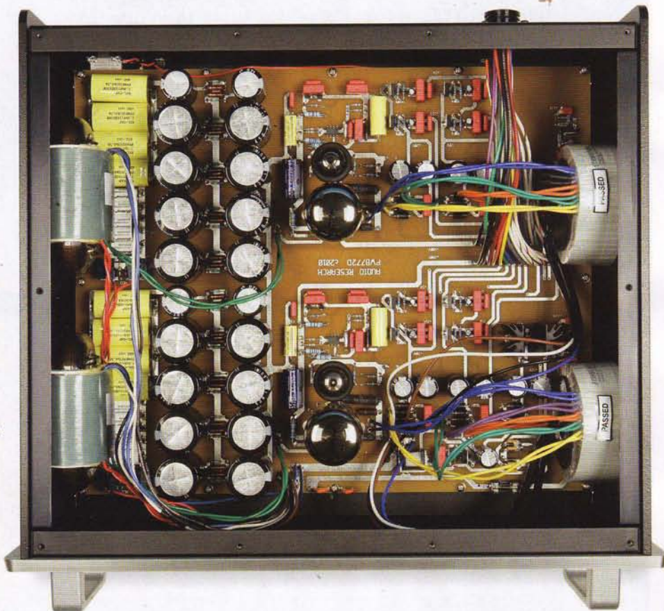
ABOVE: Housed in a separate chassis, the choke-regulated Anniversary PSU employs a pair of 6550C and 6H30P tubes per channel. The idle power consumption is around 200W
